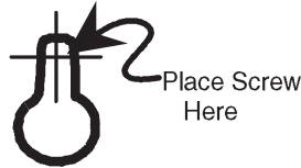
MOUNTING HOLE FOR 920 REMOTE DISPLAY
