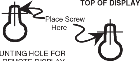
MOUNTING HOLE FOR 930 REMOTE DISPLAY
